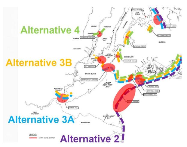
**Figure 1**: Conceptual alternative layouts showing features involving storm surge barriers (red areas) being considered in the HAT Study
